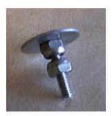
The washer is to give the bolt a good foundation in your lead
